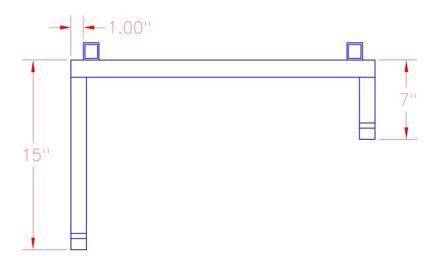
Notes: The vertical legs on the deck support will vary depending on the configuration of the mower deck used.
