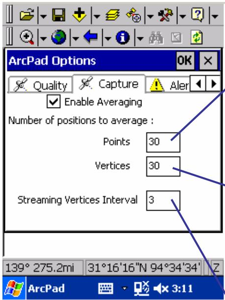
19. Tap inside the box to the right of Points to enter the number of continuous GPS fixes you want to average when capturing a point feature with your GPS receiver. Averaging multiple GPS fixes will improve the accuracy of the captured point. It is recommended that at least 20 and up to 180 GPS fixes be used when averaging points. Using the stylus and the provided keyboard, type 30.
