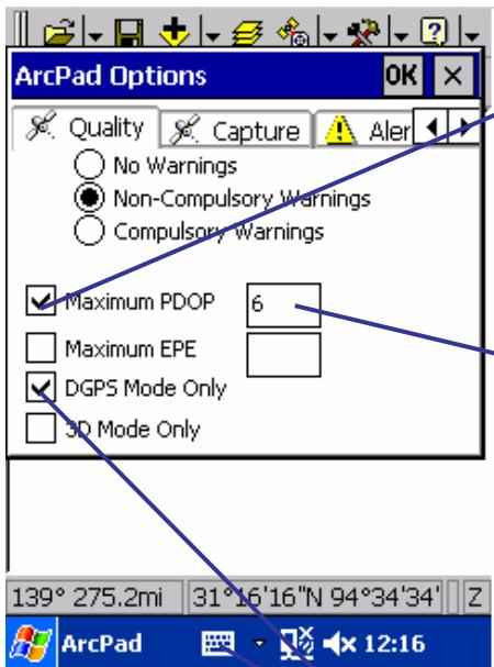
12. Tap inside the box to the left of Maximum PDOP. Position Dilution of Precision (PDOP) is the most commonly used measure of GPS accuracy. Position coordinates indicated by your GPS receiver with low PDOP values are more accurate than those indicated with high PDOP values.
