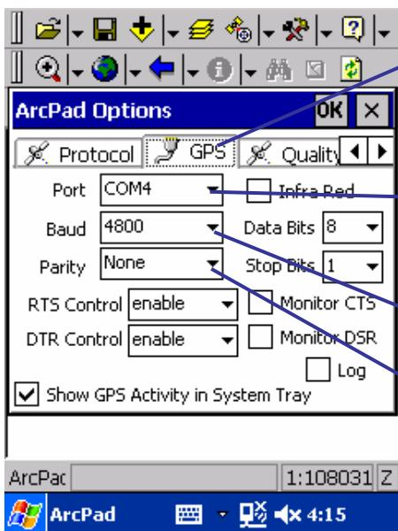
4. Tap the GPS page on the ArcPad Options dialog box to display the GPS page. The GPS page is used to specify the communication parameters of your GPS receiver.
