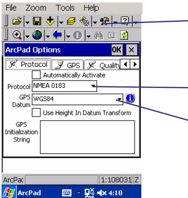
1. Tap the Tools button on the Main toolbar to open the ArcPad Options dialog box. The Protocol page is used to specify the protocol, datum and other settings of your GPS receiver.
