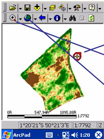
11. The GPS Cursor is displayed after the GPS receiver has been activated. The GPS Cursor is displayed at your current GPS position on the map and will move on the map as you navigate around the field.
