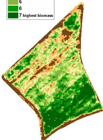
The NDVI measures the infrared reflectiveness of the vegetation which results in a color-coded image that represents an indication of plant health/vigor relative to other plants in the image. Once loaded onto a PDA, these geo-referenced images can be used by agents, producers or crop consultants to scout fields for insect and disease damage, water stress or to make variable rate applications of fertilizers and chemicals.
