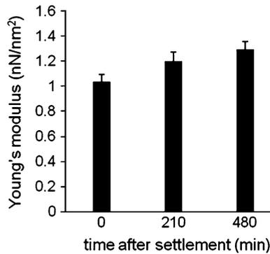
**Fig. 4** Increased Young's modulus value for ivy nanoparticles. Each point represents an average of 30 approach curves  $\pm 95\%$  confidence limits
