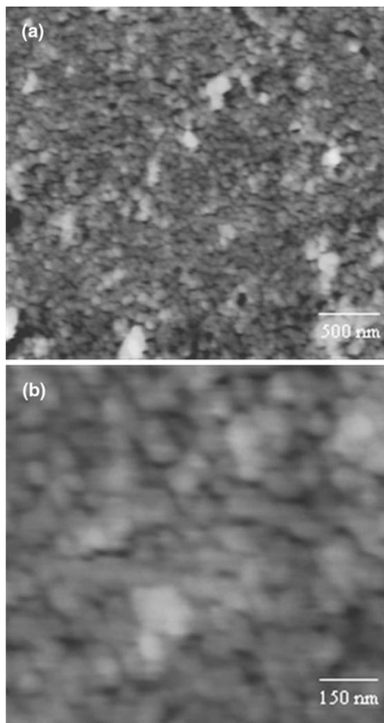
**Fig. 1** Nanoparticles released from the tip of in vitro grown ivy rootlets. AFM tapping-mode images of content from the tips of cultured ivy rootlets after 5 h of settlement. **a**  $3.3 \times 3.3$  nm scanning window. **b**  $1.0 \times 1.0$  nm scanning window
