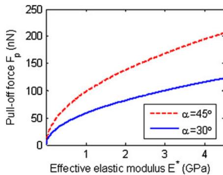
**Fig. 6** Curves from the mechanics model of adhesion force between nanoparticles and the substrate for materials with different Young's modulus and at two contact angle of  $30^\circ$  (solid line) and  $45^\circ$  (dashed line)
