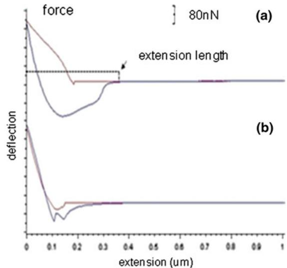
**Fig. 2** A typical approach-retract cycle illustrates the adhesion profile and other mechanical properties of ivy nanoparticles examined under AFM in **a**. Saw-toothed curves were occasionally observed in **b**
