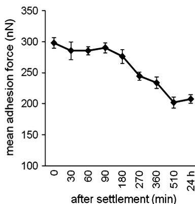
**Fig. 3** Change of adhesion force within 24 h. The force was measured at various time points after deposition. Each point represents an average of 30 retraction curves  $\pm 95\%$  confidence limits
